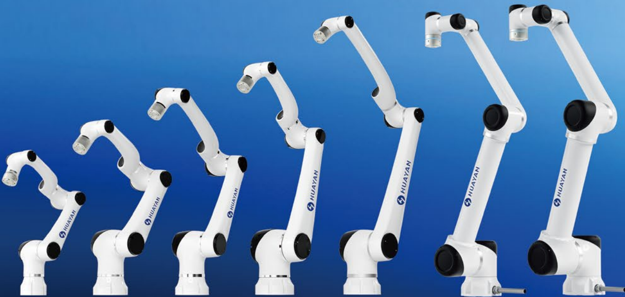
Elfin-Ex & Smart-Ex Explosion-proof Collaborative Robots
